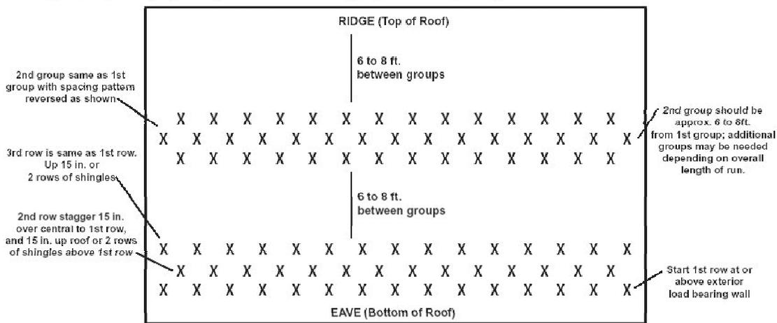
**Snow guards should never be placed beyond the bearing wall on an extended roof section. This can result in ice damming and cause structural damage**
